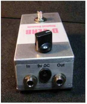
This is the D-VERB (Digital Reverb) kit. This really is an excellent reverb and is also the base of some of the reverb units being built by Hermida Engineering, used by many big name guitarists. The source of the reverb sound is a digital reverb modual made called Digi-Log<sup>™</sup> Reverb by Accutronics. Throughout this document we will refer to this modual as the "reverb brick".
