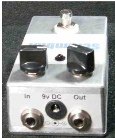
This is the Ampeg Scrambler Replica kit. This is a Fuzz/Octave unit. The Octave up sound is not as pronounced as some of the other Octave up stompboxes, but this one has a unique one-of-a-kind sound that you don't want to miss out on.
