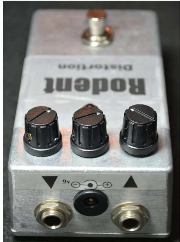
This is the Rodent Distortion kit, a replica of the ProCo™ Rat™. There were/are several versions of the Rat™. This project and kit is based on an older version of the Rat™ circuit sometimes known as version "B". It does not include a JFET on the input of the circuit as version "A" had. Experimentation has shown the input JFET does not have much effect on the sound and is probably not worth the extra parts to include in this project.
