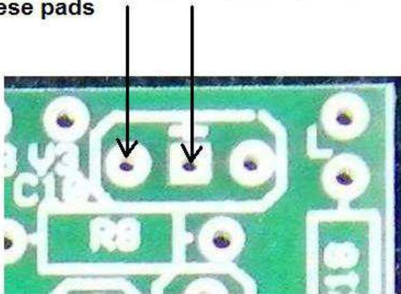
For a film non-polarized 1uF cap, use these pads
