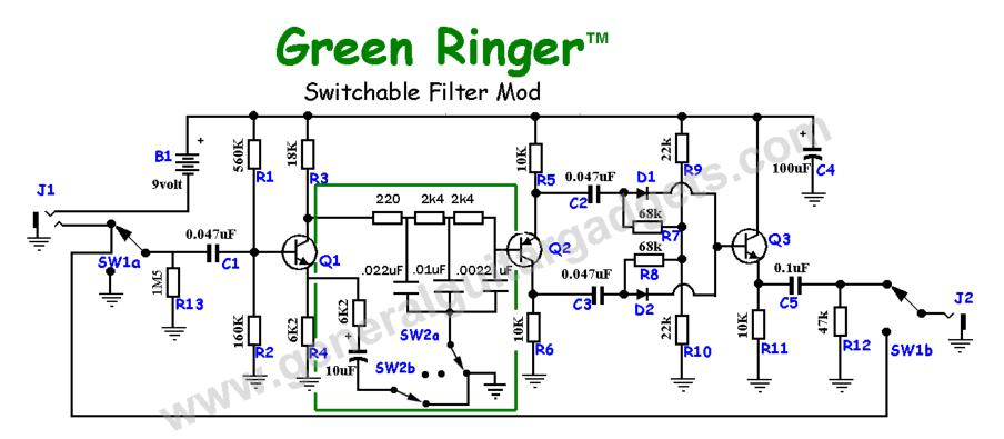
Drawn by: JD Sleep Filter Mod: Ben Milner Q1, Q3 = 2N5088 or 2N5089 Q2 = 2N3906 (low gain) D1, D2 = Diodes, matched set, SI, Ge or Schottky SW1a, SW1b - DPDT heavy duty footswitch
