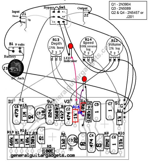
The additional LED will flash in time with the speed rate even when bypassed.
