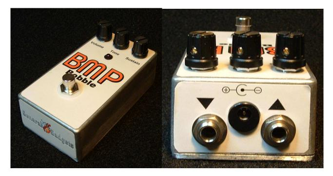
This is a replica of the **Electro-Harmonix Big Muff Pi** referred to as **BMP** in these documents. This is one of the most famous distortion pedals, described by some as violin sounding and very heavy but sustained and smooth distortion.
