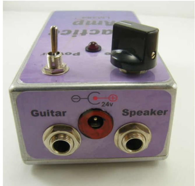
This is the instructions and notes for the **LM384** 14 pin IC Amplifier (5 watt audio power amplifier). This amplifier is also completely compatible with the **LM380** 14 pin IC 2.5 watt audio power amplifier), just be cautious about the power supply differences if you use the LM380 IC.
